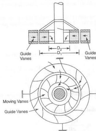
Fig.1.21 Inward flow reaction turbine
