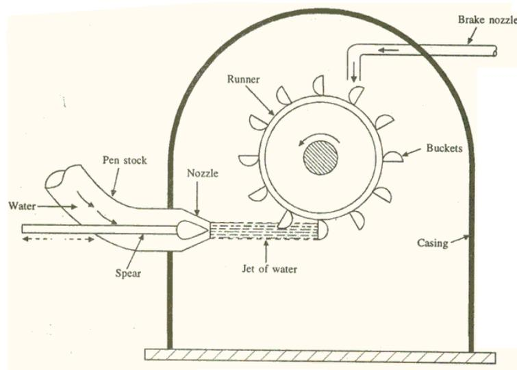
Fig. 1.19 Pelton wheel turbine
