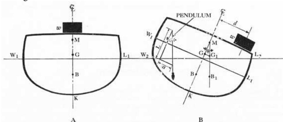
The buoyant force F<sub>b</sub> through B' and weight w through G constitute a couple acting in anti-clockwise direction and thus bringing the floating body in the original position. To determine the meta-centric height of a floating body, we know the center of gravity of floating body. Place the known weight (w) over the center of the body.
