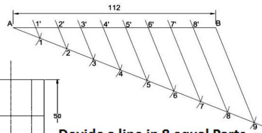
**Devide a line in 8 equal Parts**
