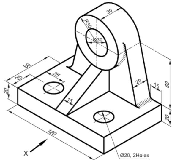
2. Pictorial view of a machine component is shown in Fig Draw following: (1) F.V. From X (2) T.V. and (3) Sectional LHSV from AA using Third Angle System
