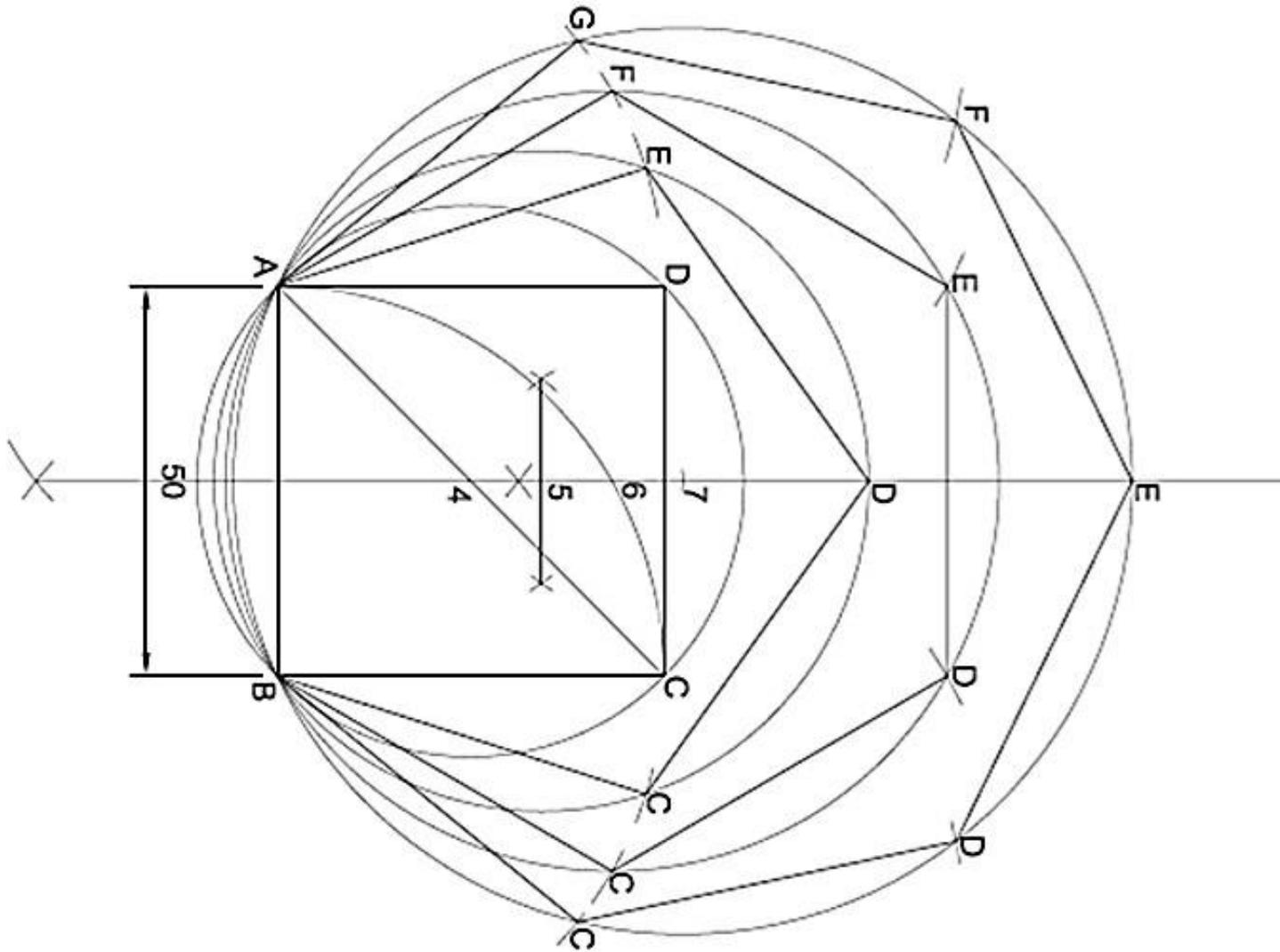
**1.12** To draw polygons using protractor. Length of side = 50mm
