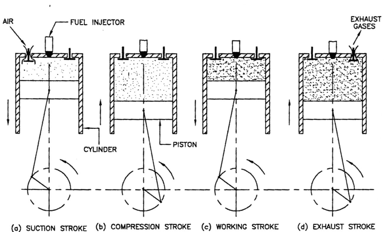
**Fig. 7.8 Four stroke diesel engine**
