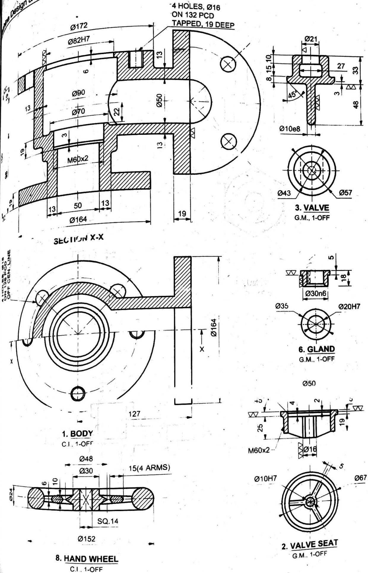
Fig. 7.35 : Steam stop valve details
