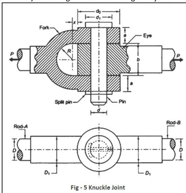
Fig - 5 Knuckle Joint
