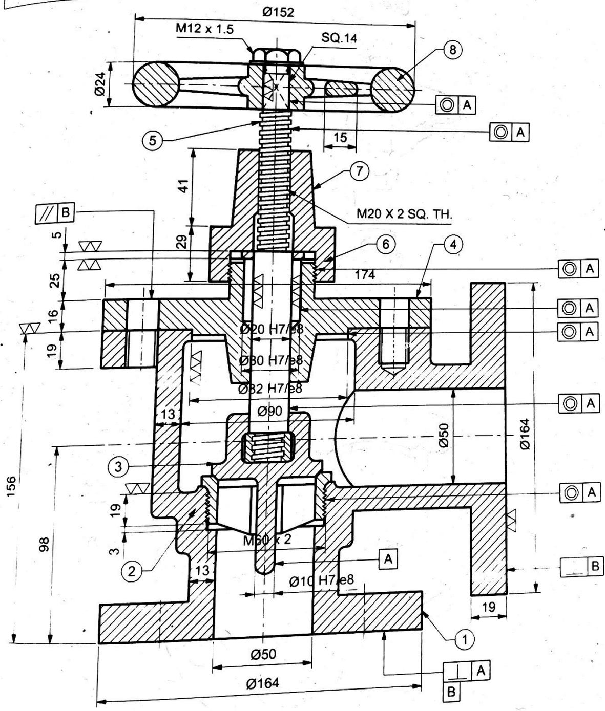
**Fig. 7.37 : Assembly of steam stop valve**
