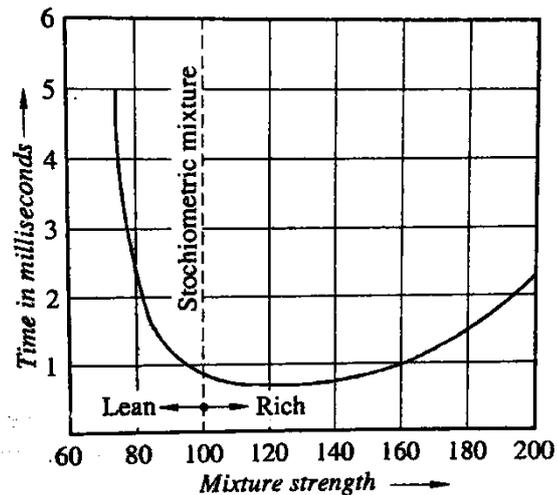
Fig. 7. 8 Effect of A/F Ratio on flame propagation
