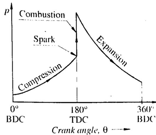
(b) theoretical  $p - \theta$  diagram with combustion
