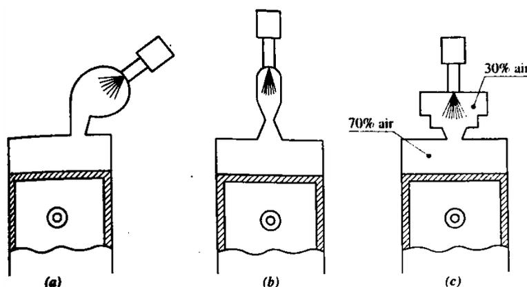
*Fig.7. 26 Precombustion chamber*
