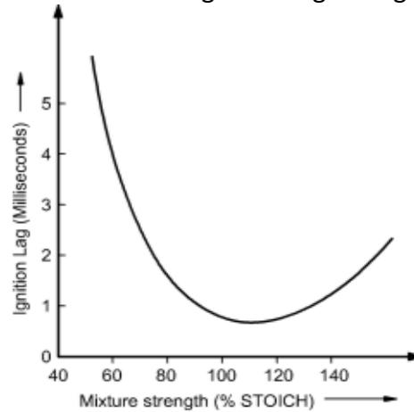
Fig.7. 5 Effect of A/F Ratio on Ignition Lag
