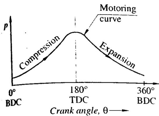
Fig. 7.2 (a)  $p - \theta$  diagram without combustion (non-firing)
