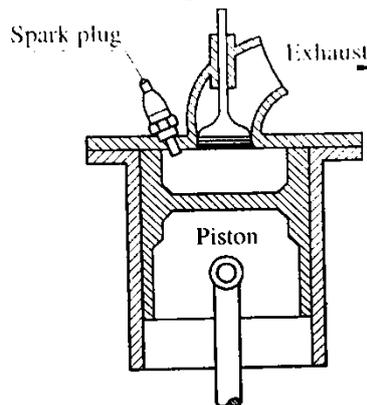
*Fig.7. 15 Rover Head Combustion Chamber*
