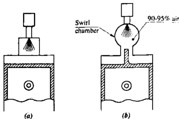
Fig.7. 27 Turbulent or Indirect Injection (IDI) Combustion Chambers
