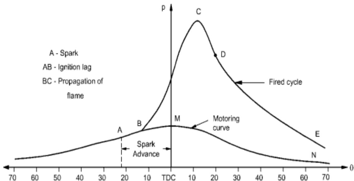
Fig 7.3 Actual  $p - \theta$  diagram for S.I. engine
