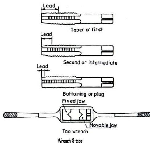
A tap is a hardened and steel tool, used for cutting internal thread in a drill hole. Hand Taps are usually supplied in sets of three in each diameter and thread size. Each set consists of a taper
