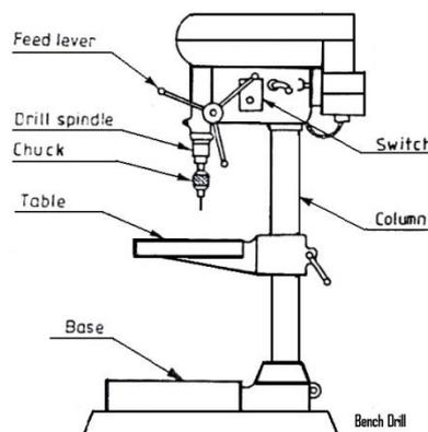
Holes are drilled for fastening parts with rivets, bolts or for producing internal thread. Bench drilling machine is the most versatile machine used in a fitting shop for the purpose. Twist drills, made of tool steel or high speed steel are used with the drilling machine for drilling holes.
