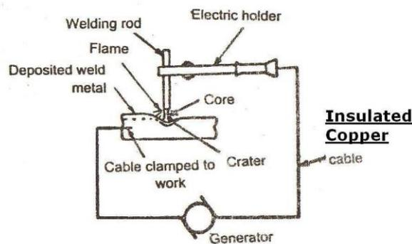
**Metal-arc Welding Circuit**
