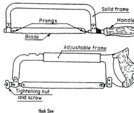
The Hack Saw is used for cutting metal by hand. It consists of a frame, which holds a thin blade, firmly in position. Hacksaw blade is specified by the number of teeth for centimeter. Hacksaw blades have a number of teeth ranging from 5 to 15 per centimeter (cm). Blades having lesser number of teeth per cm are used for cutting soft materials like aluminum, brass and bronze. Blades having larger number of teeth per centimeter are used for cutting hard materials like steel and cast Iron.
