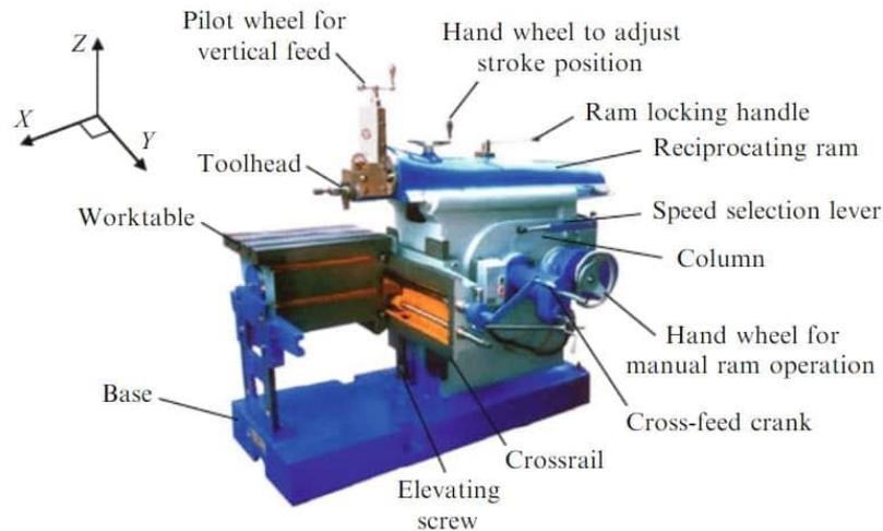
A metalworking shaper is somewhat analogous to a metalworking planer, with the cutter riding a ram that moves relative to a stationary workpiece, rather than the workpiece moving beneath the cutter. The ram is typically actuated by a mechanical crank inside the column, though hydraulically actuated shapers are increasingly used. Adding axes of motion to a shaper can yield helical tool paths, as also done in helical planing.
