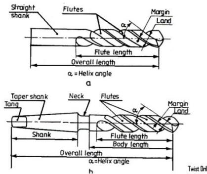
Twist drills are used for making holes. These are made of High speed steel. Both straight and taper shank twist drills are used. The parallel shank twist drill can be held in an ordinary self – centering drill check. The taper shank twist drill fits into a corresponding tapered bore provided in the drilling machine spindle.
