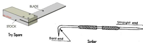
It is measuring and marking tool for 90<sup>0</sup> angle. In practice, it is used for checking the sureness of many types of small works when extreme accuracy is not required. The blade of the Try square is made of hardened steel and the stock of cast Iron or steel. The size of the Try square is specified by the length of the blade.
