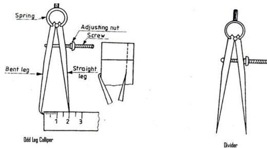
This is also called ‘Jenny Caliper’ or Hermaphrodite. This is used for marking parallel liners from a finished edge and also for locating the center of round bars; it has one leg pointed like a divider and the other leg bent like a caliper. It is specified by the length of the leg up to the hinge point.
