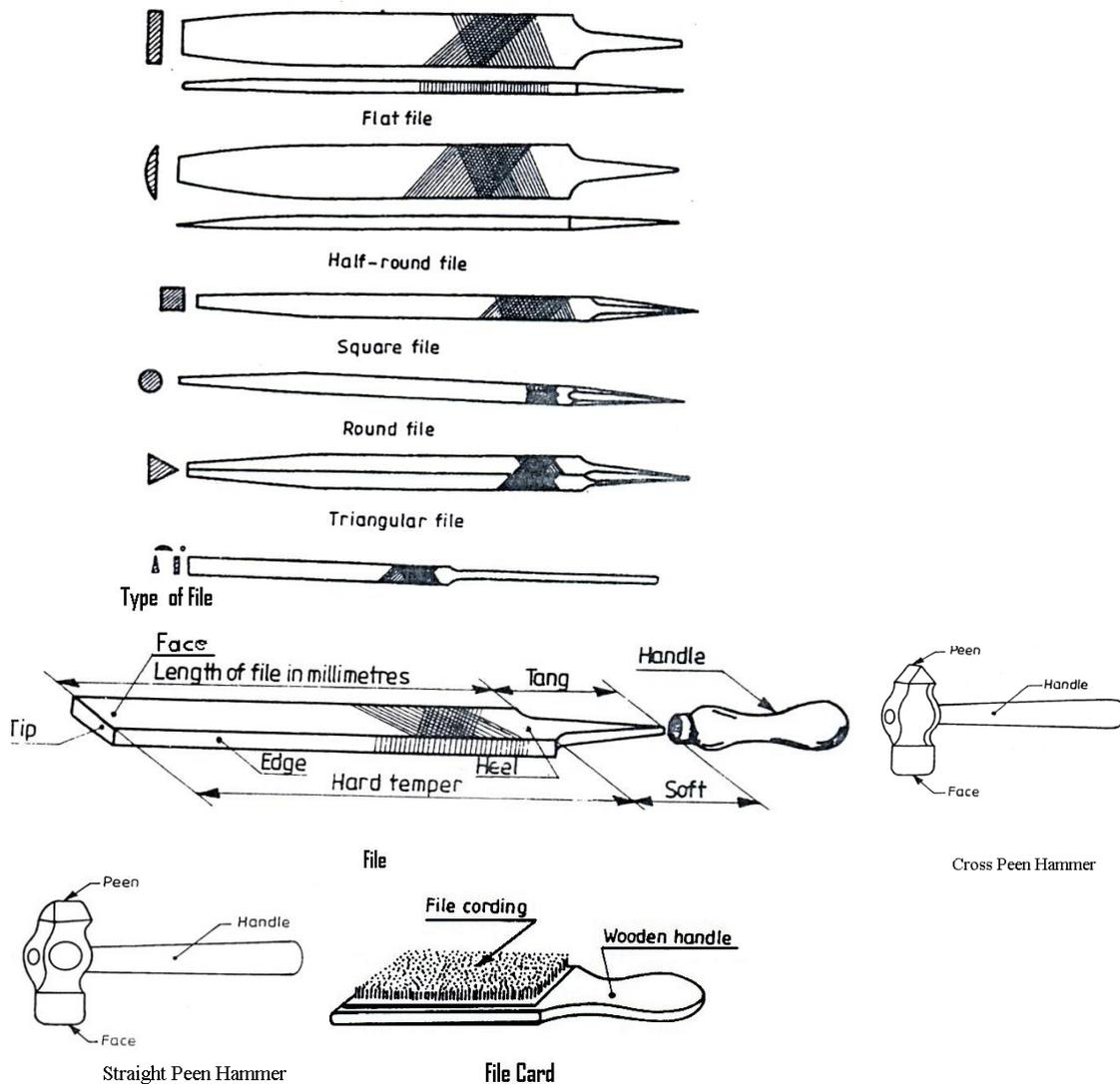
**File:** A file is a hardened piece of high grade steel with slanting rows of teeth.
