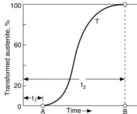
**Figure 4.10** Isothermal transformation of austenite to pearlite.
