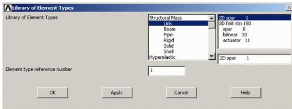
For this example, we will use the 2D spar element as selected in the above figure. Select the Element shown and click 'OK'. You should see 'Type 1 LINK1' in the 'Element Types' window. Click on 'Close' in the 'Element Types' dialog box.
